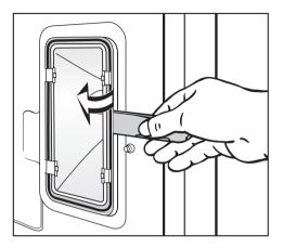
■ Use the lever to release the lamp cover from its frame.
